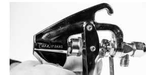
STEP 2 Tighten nut (3.3) with a 9mm spanner. While tightening make sure the lever handle still has movement.
