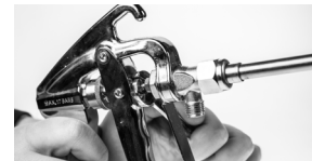
LEAKING FROM NEEDLE SHAFT Loosen nut (3.2) with a 10mm spanner.
