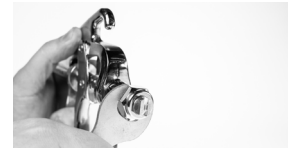
NOZZLE LEAKING When tightening make sure to use a 22mm spanner.
